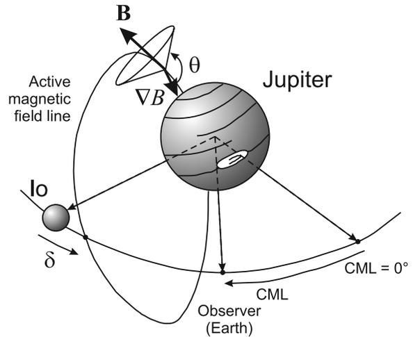
**Figure 1.** Schematic illustration of the parameters of our model. The radiation is assumed to be emitted at the local gyrofrequency along an active magnetic field line intersecting Io's wake with a lag  $\delta$ . The radio emission is beamed into a hollow cone with half-angle  $\theta$  and axis parallel to the direction of the gradient of the magnetic field modulus  $\nabla B$ .
