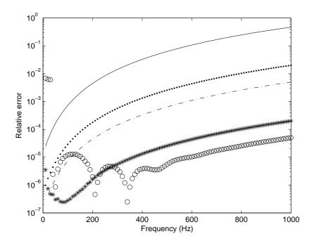
Fig. 9. Error in the Green's function versus the size of the periodic cell for the acoustic case: \_\_\_ a=b=0.05m, • a=b=0.01m, -.-. a=b=0.005m, \* a=b=0.001m, o a=b=0.0005m.
