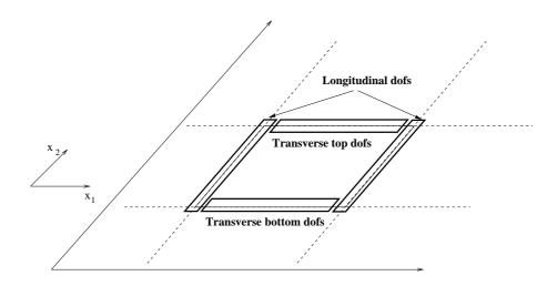
Fig. 3. Transverse and longitudinal degrees of freedom.
