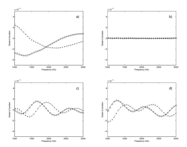
Fig. 15. Comparison of the present method and a full FEM computation for a periodic two materials medium: a) x component of displacement at point (0.25,0), b) y component of displacement at point (0.5,0.5), d) y component of displacement at point (0.5,0.5), d) y component of displacement at point (0.5,0.5), real part present method, -. imaginary part present method,  $\mathbf{o}$  real part full FEM.
