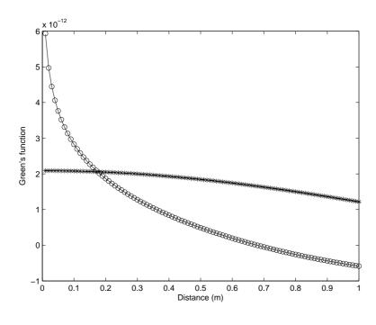
Fig. 13. Comparison of analytical and numerical Green's functions for the two-dimensional elasticity: \_\_\_\_ real part analytical, -. \_ . imaginary part analytical,  $\mathbf{x}$  real part numerical, o imaginary part numerical.
