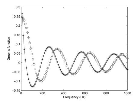
Fig. 7. Comparison of analytical and numerical Green's functions for the acoustic case: \_\_\_\_ real part analytical, -.-. imaginary part analytical, \* real part numerical, o imaginary part numerical.
