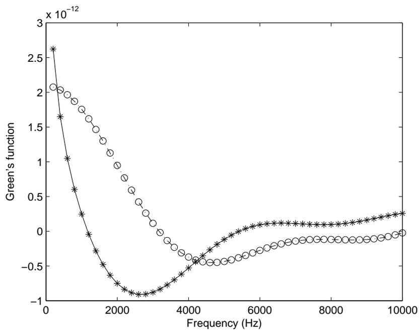
Fig. 10. Comparison of analytical and numerical Green's functions for the two-dimensional elasticity: — real part analytical, - . - . imaginary part analytical, \* real part numerical, o imaginary part numerical.
