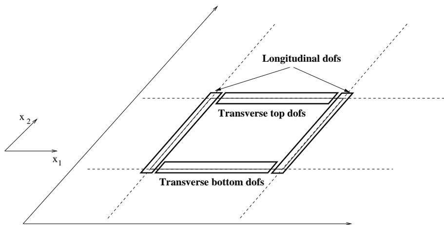
Fig. 3. Transverse and longitudinal degrees of freedom.
