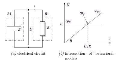
Figure 4: Interconnection of electrical components
