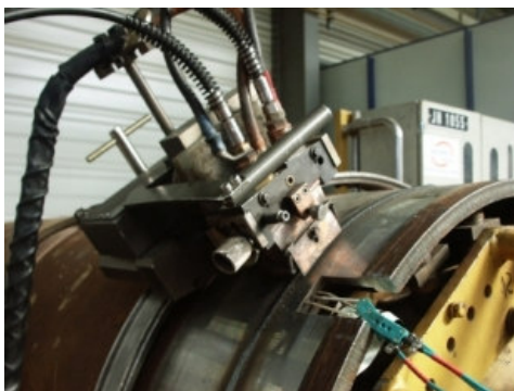
Figure 7. Temperature measurements in an actual welding operation
