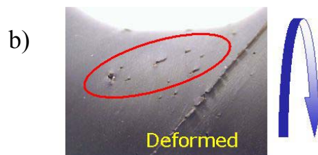
Figure 1. Dog-bone specimen a) dimensions ; b) multiple cracks under cyclic torsion
