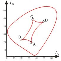
Fig 3. Singular curves and cusp points in a slice of the 3-RPR manipulator joint space  $(L_2, L_3)$  for  $L_1=34$ .
