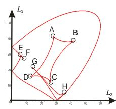
Fig 4. Singular curves and cusp points in a slice of the 3-RPR manipulator joint space  $(L_2, L_3)$  for  $L_1=27$ .
