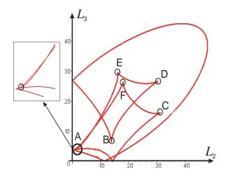
Fig 2. Singular curves and cusp points in a slice of the  $3-R\underline{P}R$  manipulator joint space  $(L_2, L_3)$  for  $L_1=14.98$ .
