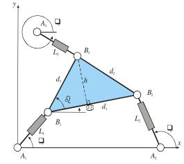
Fig 1. The 3-RPR parallel manipulator under study.
