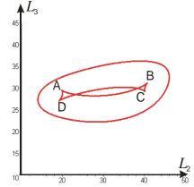
Fig 5. Singular curves and cusp points in a slice of the joint space  $(L_2, L_3)$  of the second 3-RPR manipulator studied for  $L_1=3$ .
