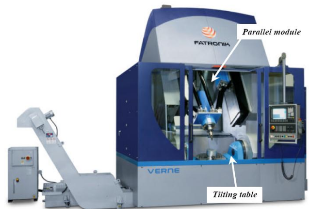
Fig. 1. Overall view of the VERNE machine
