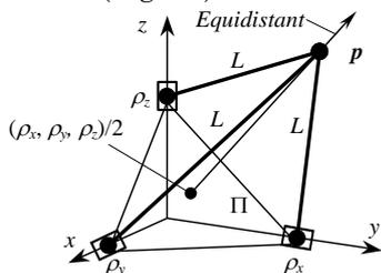
Fig. 6. Geometrical solution of the direct kinematics
