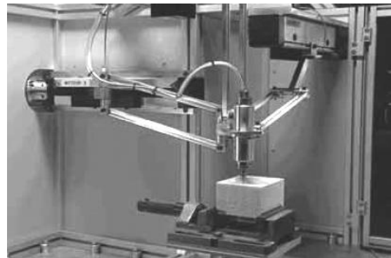
Figure 1: The Orthoglide kinematic architecture. (© CNRS Photothèque / CARLSON Leif)
