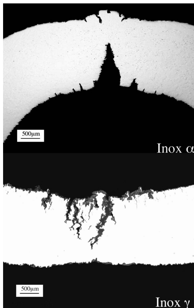
Fig. 5 - Thermal fatigue damage for ferritic (·) and austenitic (A) grades.
