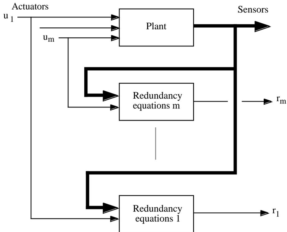
Figure 1 : actuator faults detection using unknown-input redundancy equations
