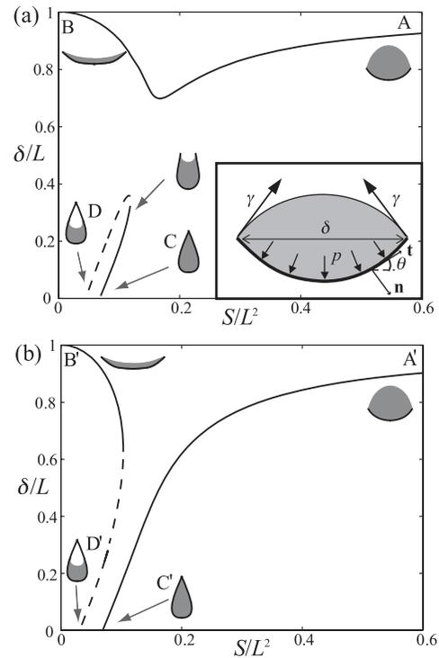
FIG. 4. Distance between the rod tips vs drop volume for different values of the rod length  $L$ : (a)  $L = 3.4L_{\text{EC}}$  reopening of the rod as  $S$  decreases; (b)  $L = 4L_{\text{EC}}$  complete wrapping of the rod around the drop. The inset shows a sketch of a 2D drop deposited on a flexible sheet.
