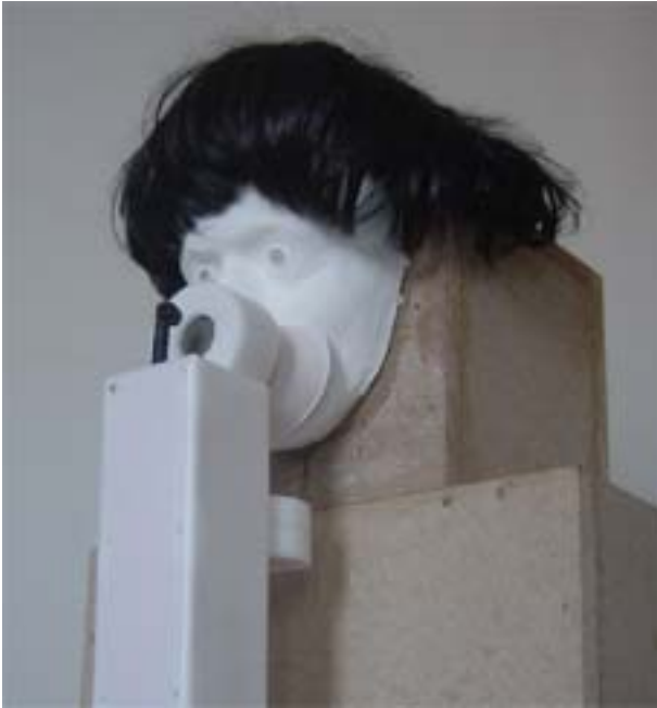
Fig 4 Artificial head loudspeaker to study acoustic distortion
