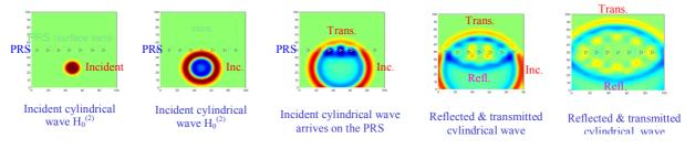
Fig. 3. Interaction between a cylindrical wave and a Partially Refflective Surface (PRS)
