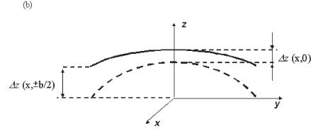
**FIGURE 7** (a) Representation of anticlastic bending of composite beam. (b) Anticlastic bending at given x along beam axis for 2 crack lengths (a and  $a+\delta a$ ). The higher, less-curved profile (continuous line) corresponds to a longer crack length and, therefore, a lower bending moment than the lower (dotted) profile.
