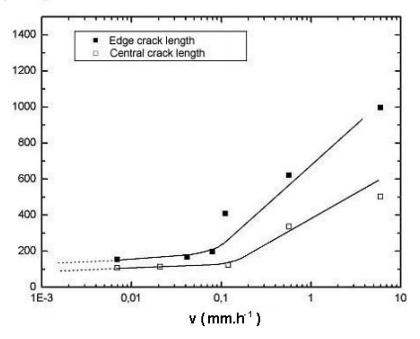
**FIGURE 5** Estimation of  $G_{IC}$  (for an aged sample) depending on whether crack length is estimated at edge or centre of composite/aluminium structure.
