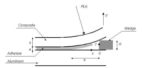
FIGURE 1 Schematic representation of wedge test with one flexible beam.
