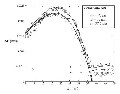
**FIGURE 11** Shifting of the composite beam, 24 h after wedge insertion with a time interval of  $\Delta t = 40\,\mathrm{min}$ : (x) experimental data for the centre line; (o) experimental data for the side line; (—) calculated for centre line; (- - -) calculated for side line.
