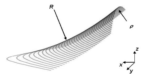
FIGURE 6 Schematic representation of anticlastic curvature.
