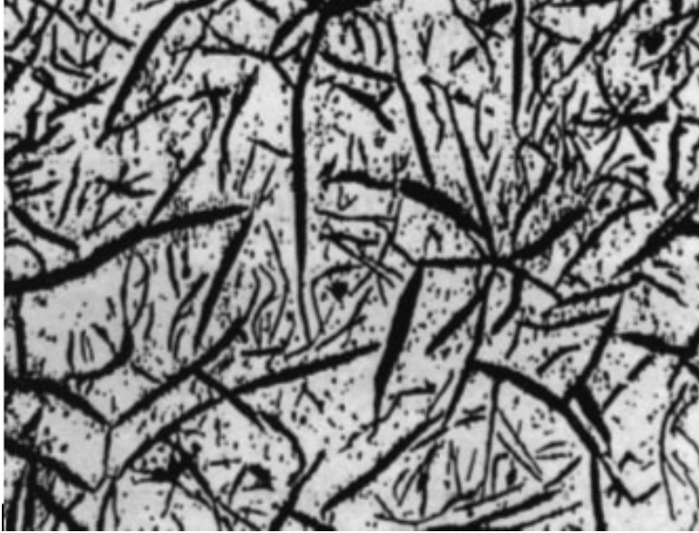
Fig. 3.11 Typical equiaxed carbon flakes in gray cast iron: optical metallography, typical size 500 \mu\text{m} .
