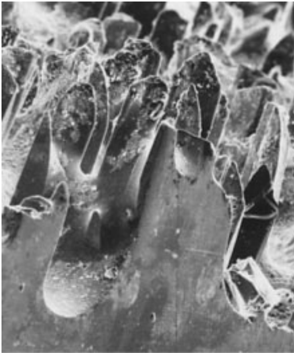
Fig. 3.10 Shape of the columnar interface of an Al 2 Cu intermetallic compound: SEM observation after quickly removing the liquid (Dupouy, 1986).
