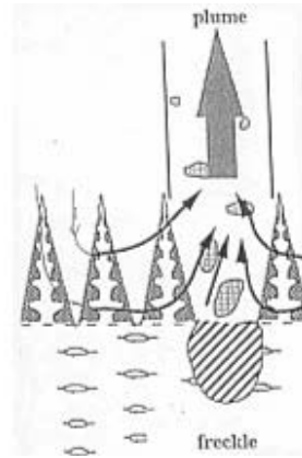
Fig. 3.46 Effect of convection on the structure of an Al–Cu alloy grown under vertically destabilized configuration: downward solidification of a hyper-eutectic alloy. One freckle appears here as a region with smaller dendrites (Dupouy and Camel 2000).
