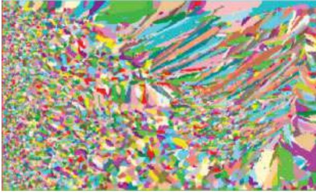
Fig. 3.38 Grain structure of an alloy as predicted by Gandin's stochastic model (Gandin and Rappaz, 1994). The growth proceeds from the left to the right and the effect of melt convection can be seen. The colors are representations of the various crystallographic orientations of the grains.
