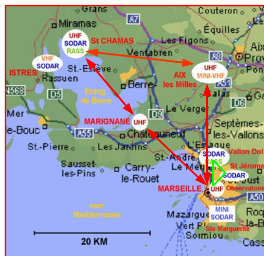
Figure 1. The UHF wind profiler network deployed during ESCOMPTE campaign. Sodar and VHF profilers locations are also shown.
