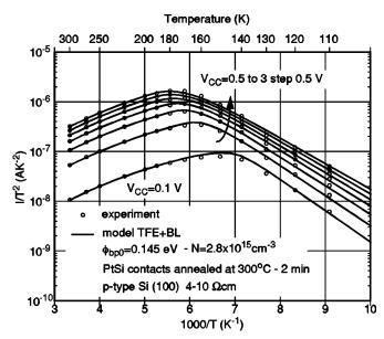
FIG. 11. Experimental and calculated Arrhenius plot using the thermionic field emission (TFE) transport model including barrier lowering (BL) due to image charge induction. Optimum model parameters are  $\phi_{bp0}=0.145$  eV,  $N=2.8\times10^{15}$  cm<sup>-3</sup>,  $R_{\rm Si}=98$   $\Omega$ , and  $\alpha=1.5$ .
