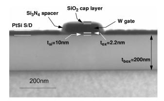
FIG. 14. TEM cross section of *p*-type SB-MOSFET with PtSi S/D. This device architecture features a thin, 10 nm thick SOI channel, a 2.2 nm  $SiO_2$  gate oxide, a 40 nm thick tungsten gate encapsulated by 15 nm wide  $Si_3N_4$  spacers at each side wall, and a deposited  $SiO_2$  capping layer on the top.
