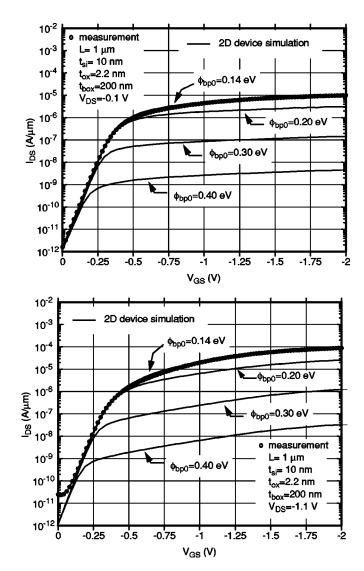
FIG. 16. Comparison between measured and simulated  $I_{DS}$ - $V_{GS}$  characteristics of a long channel *p*-type SB-MOSFET with PtSi S/D: (a)  $V_{DS}$ = -0.1 V; (b)  $V_{DS}$  = -1.1 V. Simulations account for a variable zero-field Schottky barrier  $\phi_{bp0}$  (0.14, 0.2, 0.3 0.4 eV). A correct current performance is achieved for the lowest barrier (0.14 eV), which consistently corresponds to the value (0.145 eV) that best fits the Arrhenius plot measured on test structures.
