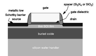
FIG. 1. Schematic representation of a MOSFET that integrates a low Schottky barrier source/drain.
