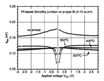
FIG. 8. Voltage dependence of the effective Schottky barrier to holes measured on Pt–Si Schottky junctions. The extraction of  $\phi_{bp0}$  is based on an activation energy method performed at low temperature and in reverse mode.
