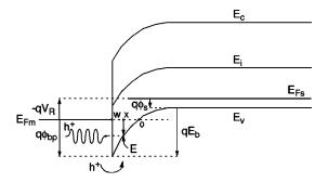
FIG. 9. Band bending at Schottky interface for a reverse bias. This diagram is representative of hole tunneling with energy *E* crossing the barrier at location *x*. When  $E > E_b = q(\phi_b - \phi_s + V_R)$  thermionic emission is enabled.
