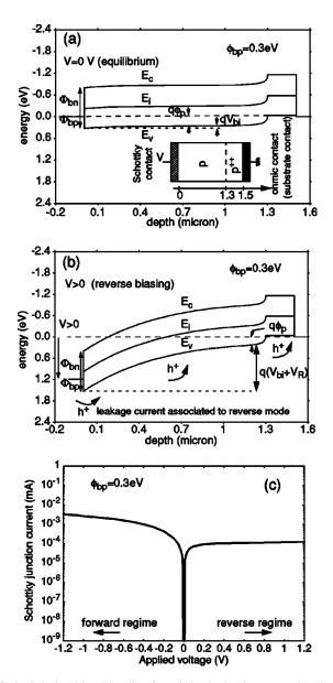
FIG. 3. Calculated band bending for a Schottky barrier on a *p*-doped substrate. The Schottky barrier to holes  $\phi_{bp} = 0.3$  eV remains representative of a relatively low barrier (a) at equilibrium, the depletion condition is not fulfilled; (b) under reverse bias, the low Schottky barrier to holes enables a large reverse current; (c) current-voltage characteristic.
