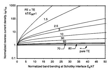
FIG. 10. Normalized reverse current as a function of the normalized band bending. A large ratio  $kT/E_{00}$  indicates that current is governed by TE, while a small value of the same ratio indicates that tunneling dominates (FE).
