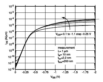
FIG. 15. Measured  $I_{DS}$ - $V_{GS}$  characteristics of a long channel *p*-type SB-MOSFET with PtSi S/D. The gate length *L* and width *W* are 1 and 10  $\mu$ m, respectively. A near-ideal subthreshold swing of 62 mV/dec is obtained. The midgap work function provided by the tungsten gate gives a threshold voltage of 0.37 V.
