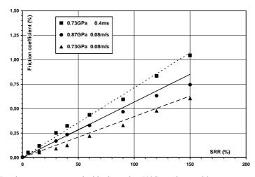
Figure 4: Traction curves measured with glycerol at 50°C, steel - sapphire contact.
