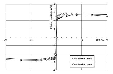
Figure 1: Low traction values given by linear paraffinic mineral base oil (LP) at 40°C.
