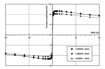
Figure 2: Typical high friction results obtained with a traction fluid (Santotrac 50, 25°C)
