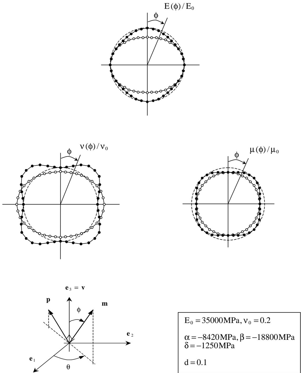
**Figure 3.** Generalized elastic moduli normalized by their initial values of a concrete weakened by a single set of parallel microcracks of unit normal  $\mathbf{v}$  (—○— open microcracks, —●— closed microcracks, --- unit circle).
