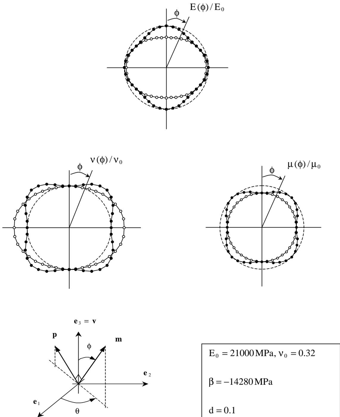
**Figure 2.** Generalized elastic moduli normalized by their initial values of a sandstone weakened by a single set of parallel microcracks of unit normal  $\mathbf{v}$  (—○— open microcracks, —●— closed microcracks, --- unit circle).
