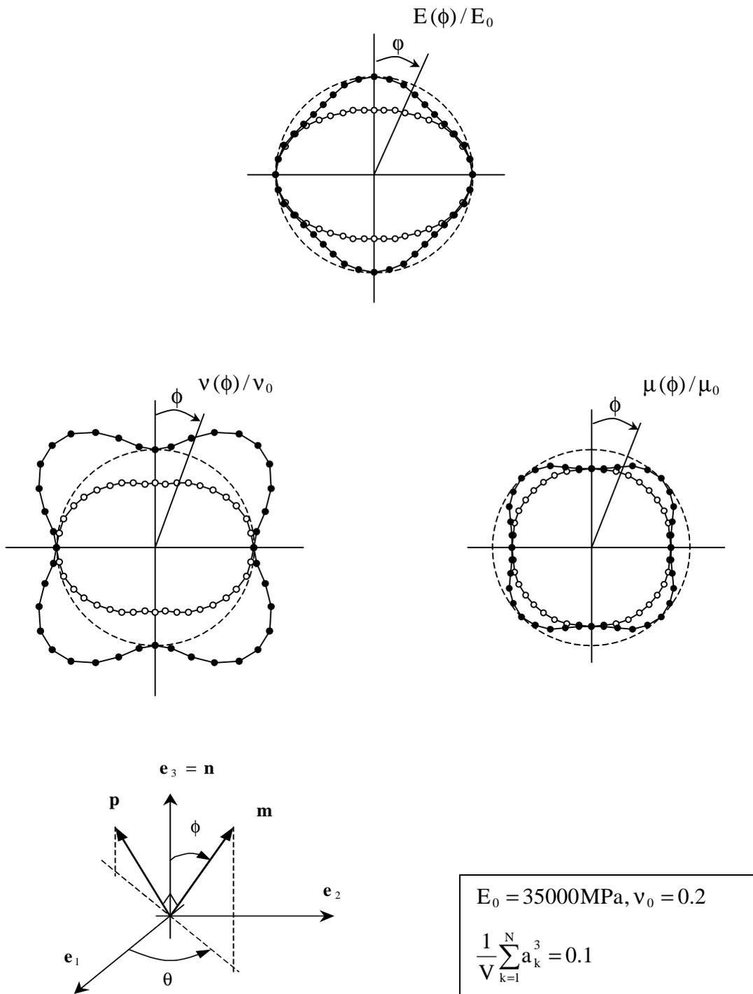
**Figure 1.** Generalized elastic moduli normalized by their initial values of a concrete weakened by a single array of parallel microcracks of unit normal  $\mathbf{n}$  (—○— open microcracks, —●— closed microcracks, --- unit circle).
