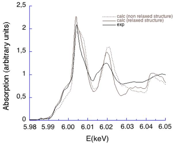
FIG. 4: Cr K-edge XANES spectra in  $\text{MgAl}_2\text{O}_4: \text{Cr}^{3+}$ . The experimental signal (thick line) is compared with the theoretical spectra calculated in the relaxed structure (solid line) and in the non-relaxed structure (dotted line)
