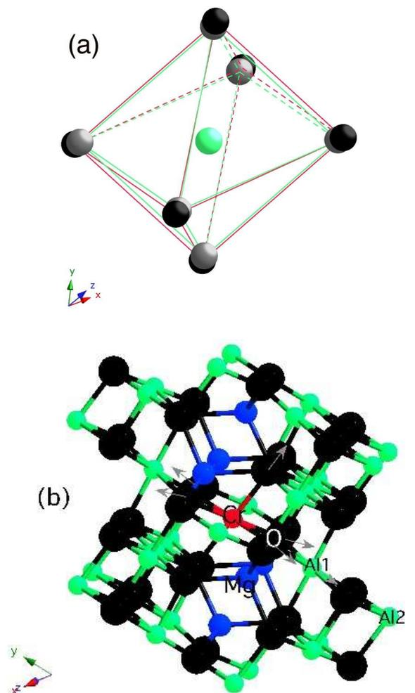
FIG. 3: (color online) (a) Cr-centred octahedron before relaxation (green) and after (red). (b) Model of structural distortions around Cr (red) in MgAl<sub>2</sub>O<sub>4</sub>: Cr<sup>3+</sup>. The O first neighbors (black) and the Al1 (green) second neighbors are displaced outward the Cr dopant in the direction of arrows.
