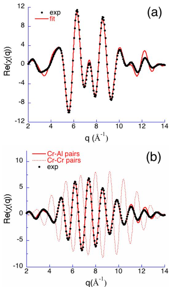
FIG. 2: (a) Inverse-FT of EXAFS data (dots) and fitted signal (solid line) for  $R=1.0-3.1$  Å. (b) Inverse-FT of EXAFS data (dots) for  $R=2.0-3.1$  Å, multi-shell fit with Cr-Al pairs (solid line) and theoretical function with Cr-Cr pairs (dashed line) in the same structural model.
