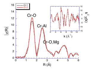
FIG. 1: Fourier-transform of k<sup>3</sup>-weighted EXAFS function for Cr-1 and Cr-2 samples (dashed and solid lines respectively). Inset: background-subtracted data
