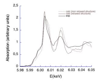
FIG. 4: Cr K-edge XANES spectra in  $MgAl_2O_4$ : Cr<sup>3+</sup>. The experimental signal (thick line) is compared with the theoretical spectra calculated in the relaxed structure (solid line) and in the non-relaxed structure (dotted line)
