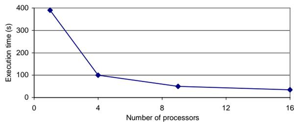
Fig.4. LU decomposition for the computation of 3D microstrip discontinuities (21408 dof) [11].
