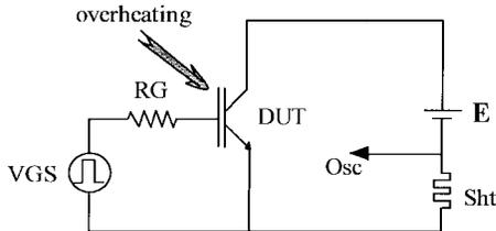
Fig. 4. Experimental circuit used for thermosensitive parameters calibration.
