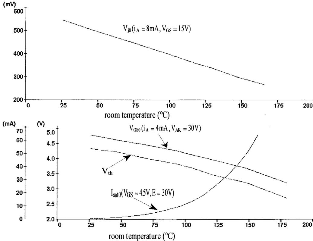
Fig. 3. Experimental calibration curves of estimated PN junction voltage ( $V_{j0}$ ), estimated gate-to-source voltage ( $V_{GS0}$ ), calculated threshold voltage ( $V_{th}$ ), and saturation current ( $I_{sat0}$ ).
