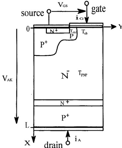
Fig. 2. Schematic diagram of IGBT under test.
