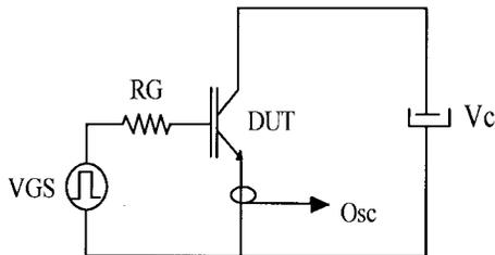
Fig. 17. Experimental circuit used for short-circuit test.
