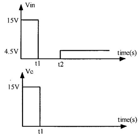
Fig. 7. Input waveforms for  $T1$  and  $T2$  switches used in the experimental circuit of Figs. 5 and 6.
