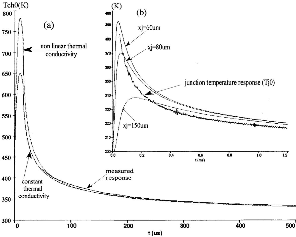
Fig. 12. (a) Heat-diffusion equation model responses with a nonlinear ( $L = 668 \mu m$  and  $S = 9.5 \text{ mm}^2$ ) and constant thermal conductivity ( $L = 597 \mu m$  and  $S = 8 \text{ mm}^2$ ). (b) HDE model responses at different abscissa  $x$  with a nonlinear thermal conductivity.
