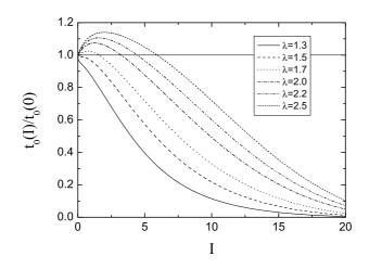
FIG. 8: The ratio  $t_G(I)/t_G(0)$  as a function of the ionicity at different values of  $\lambda$  ( $\eta = \eta_c$ ).
