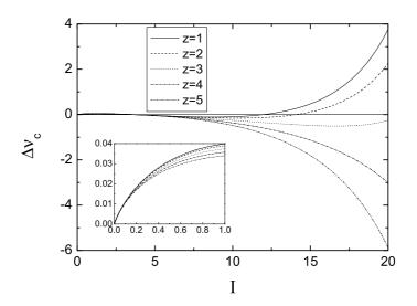
FIG. 2:  $\Delta \nu_c$  as a function of  $\mathcal{I}$  calculated from (44) for different values of z ( $\eta = \eta_c$ ). The inset depicts the behavior of  $\Delta \nu_c$  close to the origin.
