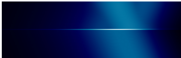
Figure 7: Modulus of the field for a symmetrical slab with \epsilon_1 = \epsilon_3 = 9 , \mu_1 = \mu_3 = 1 , \epsilon_2 = -1.5 , \mu_2 = -1 . and h = 1.3\lambda using a gaussian incident beam with a waist of 20\lambda and an incidence angle of \theta = 22.78 . The pole corresponding to the leaky mode is located at \alpha_p = (1.16823 - 0.01125i)k_0
