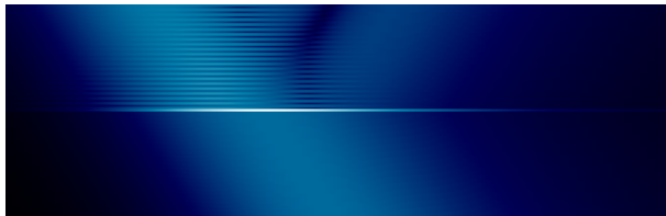
Figure 6: Modulus of the field for a symmetrical slab with \epsilon_1 = \epsilon_3 = 9 , \mu_1 = \mu_3 = 1 , \epsilon_2 = 1.5 , \mu_2 = 1 and h = 1.3 \lambda using a gaussian incident beam with a waist of 20 \lambda and an incidence angle of \theta = 22.78 .
