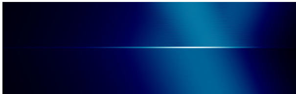
Figure 4: Modulus of the field for a symmetrical slab with \epsilon_1 = \epsilon_3 = 9 , \mu_1 = \mu_3 = 1 , \epsilon_2 = -1.5 , \mu_2 = -1 . and h = 1.3\lambda using a gaussian incident beam with a waist of 20\lambda and an incidence angle of \theta = 22.78 . The pole corresponding to the leaky mode is located at \alpha_p = (1.16823 - 0.01125i)k_0
