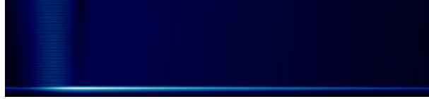
Figure 7: Modulus of the field for a left-handed slab with \epsilon_1 = 9, \epsilon_3 = \mu_1 = \mu_3 = 1, \epsilon_2 = -0.5, \mu_2 = -1.5 and h = 0.6\lambda using a gaussian incident beam with a waist of 20\lambda and an incidence angle of \theta = 21.496 . The pole corresponding to the leaky mode is located at \alpha_p = (1.0993 + 0.001267i)k_0 .
