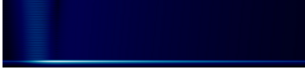
Figure 7: Modulus of the field for a left-handed slab with \epsilon_1 = 9, \epsilon_3 = \mu_1 = \mu_3 = 1, \epsilon_2 = -0.5, \mu_2 = -1.5 and h = 0.6\lambda using a gaussian incident beam with a waist of 20\lambda and an incidence angle of \theta = 21.496^\circ . The pole corresponding to the leaky mode is located at \alpha_p = (1.0993 + 0.001267i)k_0 .
