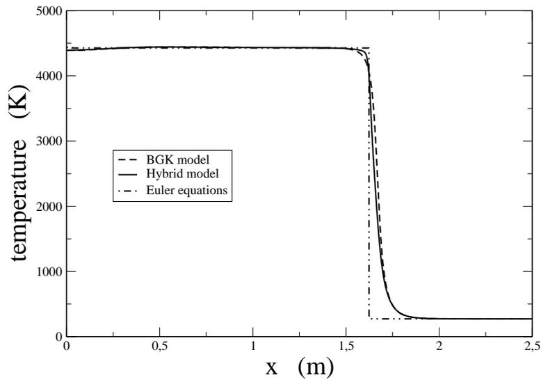
Figure 18: Unsteady shock: Temperature as a function of the space variable  $x \in [0, 2.5]$  m. Comparison between the BGK model (dashed line), the hybrid model (continuous) and the Euler equations (dashed and dotted line).
