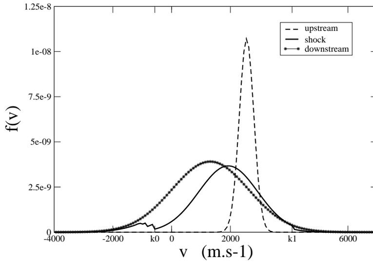
Figure 4: Stationary shock: Distribution functions as functions of the velocity  $v \in [v_{min}, v_{max}]$ . The Mach number of the flow is 6. Distribution functions upstream the shock ( $x = 0.1 m$ ) (dashed line), inside the shock ( $x = 0.5 m$ ) (continuous line) and downstream the shock ( $x = 0.9 m$ ) (stars) are presented.  $B_1 = [k_0, k_1]$  is the fluid zone at  $x = 0.5 m$ .
