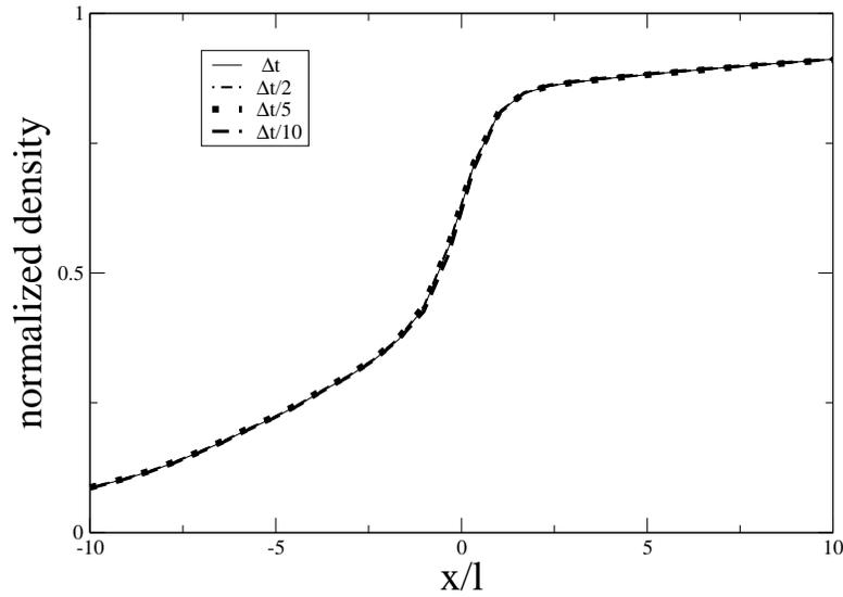
Figure 9: Stationary shock: Influence of the time step on the normalized mass density as a function of  $x/l$ ,  $x \in [0, L]$ . The Mach number of the flow is 6. Results obtained with  $\Delta t$  (continuous),  $\Delta t/2$  (dashed and dotted line),  $\Delta t/5$  (dotted line) and  $\Delta t/10$  (thick dashed line) are presented ( $\Delta t = 6 \times 10^{-7}$ ).
