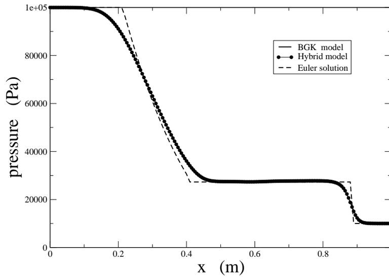
Figure 15: Sod shock tube problem: Pressure as a function of  $x \in [0, L]$ . Comparison between the BGK model (continuous), the hybrid model (circles) and the exact solution of the Euler equations (dashed line).
