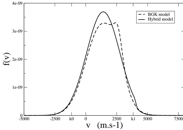
Figure 6: Stationary shock wave: Distribution functions as functions of the velocity  $v \in [v_{min}, v_{max}]$ . The Mach number of the flow is 6. The distribution functions at  $x = 0.54 m$  are represented. Comparison between the full BGK model (dashed line) and the hybrid model (continuous).
