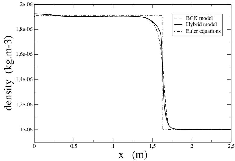
Figure 16: Unsteady shock: Mass density as a function of the space variable  $x \in [0, 2.5] m$ . Comparison between the BGK model (dashed line), the hybrid model (continuous) and the Euler equations (dashed and dotted line).
