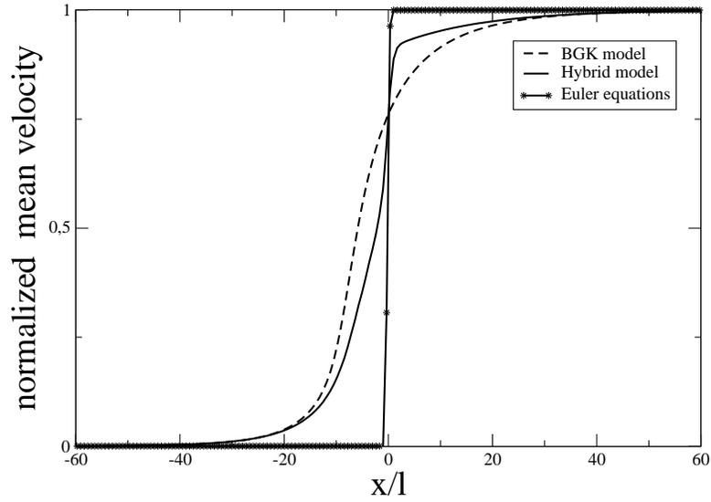
Figure 2: Stationary shock: Normalized mean velocity as a function of  $x/l$ ,  $x \in [0, L]$ . The Mach number of the flow is 6. Comparison between the BGK model (dashed line), the hybrid model (continuous) and the Euler equations (stars).
