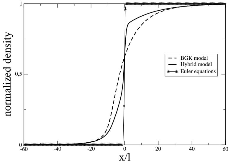
Figure 1: Stationary shock: Normalized mass density as a function of  $x/l$ ,  $x \in [0, L]$ . The Mach number of the flow is 6. Comparison between the BGK model (dashed line), the hybrid model (continuous) and the Euler equations (stars).
