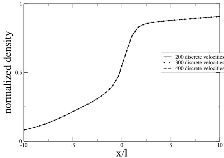
Figure 7: Stationary shock: Influence of the number of discrete velocities on the normalized mass density as a function of  $x/l$ ,  $x \in [0, L]$ . The Mach number of the flow is 6. Results obtained with 100 (continuous line), 200 (dotted line) and 400 discrete velocities (dashed line) are presented.
