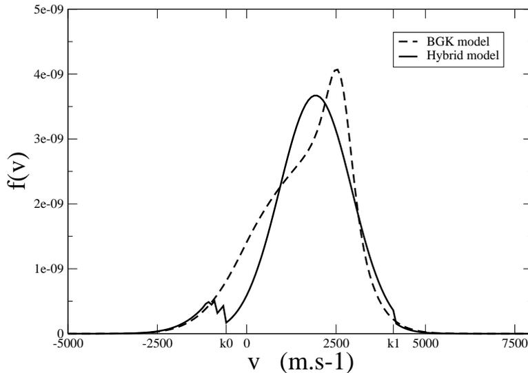
Figure 5: Stationary shock: Distribution functions as functions of the velocity  $v \in [v_{min}, v_{max}]$ . The Mach number of the flow is 6. Distribution functions within the shock ( $x = 0.5 m$ ). Comparison between the full BGK model (dashed line) and the hybrid model (continuous).  $B_1 = [k_0, k_1]$  is the fluid zone at  $x = 0.5 m$ .
