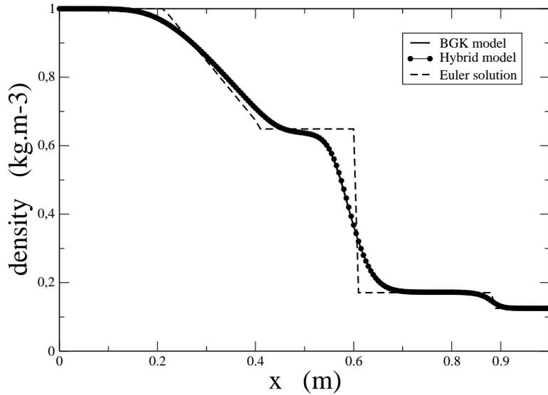
Figure 13: Sod shock tube problem: Mass density as a function of  $x \in [0, L]$ . Comparison between the BGK model (continuous), the hybrid model (circles) and the exact solution of the Euler equations (dashed line).
