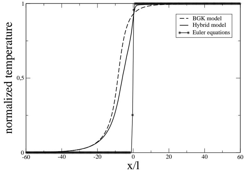
Figure 3: Stationary shock: Normalized temperature as a function of  $x/l$ ,  $x \in [0, L]$ . The Mach number of the flow is 6. Comparison between the BGK model (dashed line), the hybrid model (continuous) and the Euler equations (stars).
