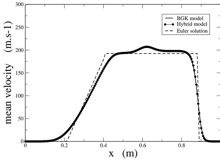
Figure 14: Sod shock tube problem: Mean velocity as a function of  $x \in [0, L]$ . Comparison between the BGK model (continuous), the hybrid model (circles) and the exact solution of the Euler equations (dashed line).
