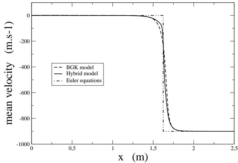
Figure 17: Unsteady shock: Mean velocity as a function of the space variable  $x \in [0, 2.5] m$ . Comparison between the BGK model (dashed line), the hybrid model (continuous) and the Euler equations (dashed and dotted line).
