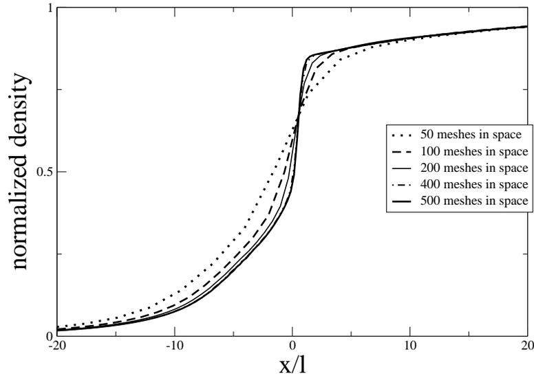
Figure 8: Stationary shock: Influence of the space discretization on the normalized mass density as a function of  $x/l$ ,  $x \in [0, L]$ . The Mach number of the flow is 6. Results obtained with 50 (dotted line), 100 (dashed line), 200 (continuous), 400 (dashed and dotted line) and 500 mesh points (thick continuous line) are presented.
