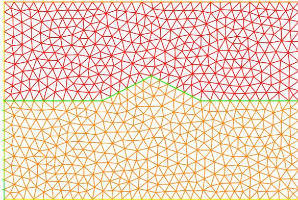
**Figure 4.** The computation domain and the initial mesh
