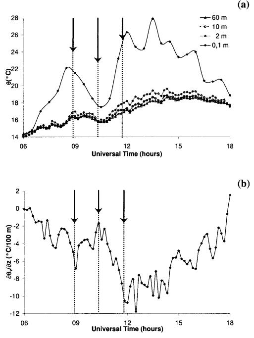
*Figure 4.* Potential temperature evolution during the eclipse day (a) from mast sensors at 0.1, 2, 10 and 60 m height and evolution of  $\partial \theta_v / \partial z$  (b) between 2 and 10 m height. Arrows have the same meaning as in Figure 2.
