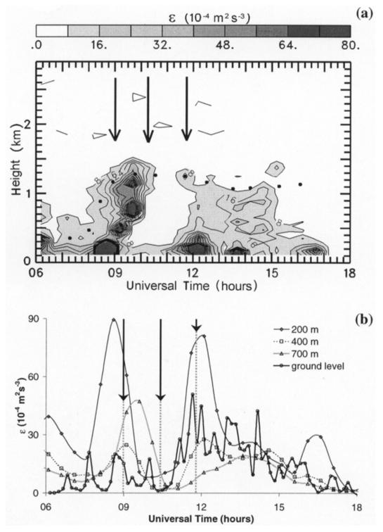
*Figure 11.* Evolution of the turbulent kinetic energy dissipation rate from the UHF radar: Time-height diagram (a) and time series (b) at 200, 400 and 700 m height. Ground level data are inferred from mast measurements at 10 m. Dots in (a) have the same meaning as in Figure 6. Arrows have the same meaning as in Figure 2.
