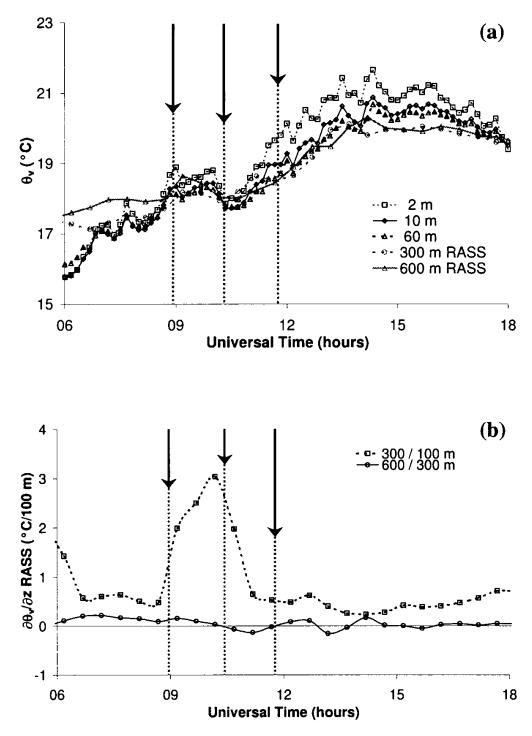
*Figure 9.* (a) Evolution of the virtual potential temperature from mast sensors at 2, 10 and 60 m height and from RASS at 300 and 600 m height (b); evolution of  $\partial \theta_v / \partial z$  between 100 and 300 m and between 300 and 600 m height (RASS measurements). Arrows have the same meaning as in Figure 2.
