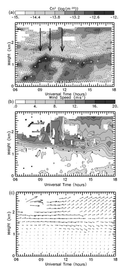
*Figure 6.* Reflectivity (a), wind speed (b), and wind direction (c) evolution inferred from the UHF radar. Dots indicate the top of the convective boundary layer inferred from (a). Arrows have the same meaning as in Figure 2.
