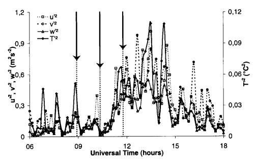
*Figure 5.* Evolution of the variances of the three wind components and the temperature (the scale is on the right for this term). Arrows have the same meaning as in Figure 2.
