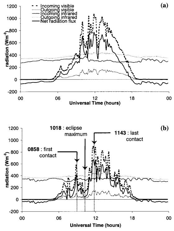
*Figure 2.* Evolution of the net radiation flux and is components for (a) a reference day (14 August 1999), and (b) for the eclipse day (11 August 1999). In (b), the first arrow represents the first contact of the eclipse, the second one the maximum obscuration, and the third one the last contact of the eclipse.
