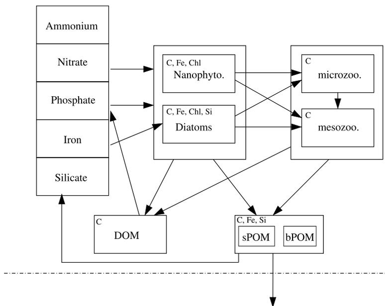
**Figure 1.** Schematic description of the PISCES ecosystem model. Not all the flows between the different compartments are drawn. The elements listed in the upper left corner of the boxes represent the explicitly modeled currencies in each pool.
