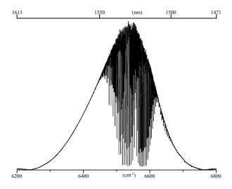
Fig. 2: Overtone spectrum of the acetylene molecule in the 1.5  $\mu$ m region demonstrating the spectral bandwidth and signal-to-noise ratio capabilities of this spectrometric technique. The strongest spectral features are the *P* and *R* branches of the  $\nu_1 + \nu_3$  band of  $^{12}C_2H_2$ .
