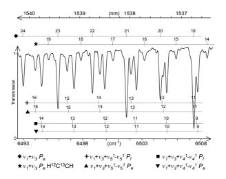
Fig. 3: Restricted portion of the spectrum shown on Fig. 2 exhibiting rotational lines of the P branches of the  $v_1+v_3$  cold band,  $v_1+v_3+v_4^1-v_4^1$  and  $v_1+v_3+v_5^1-v_5^1$  hot bands of  $^{12}C_2H_2$  [16] and the  $v_1+v_3$  cold band of  $^{12}C^{13}CH_2$ .
