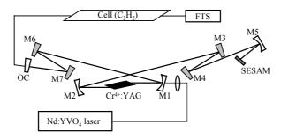
Fig. 1. Schematic of the experiment. The Cr<sup>4+</sup>YAG femtosecond laser probes a cell filled with acetylene and the resulting radiation is analysed by a Fourier transform spectrometer (FTS).
