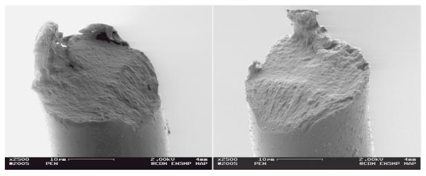
Figure 10 Complementary failure morphologies, PEN fibre, tensile failure.
