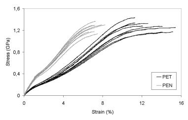
Figure 4 Stress-strain curves from tensile tests, PET & PEN single fibres.
