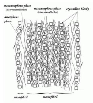
Figure 16 Fibrillar model for PET fibres [19].
