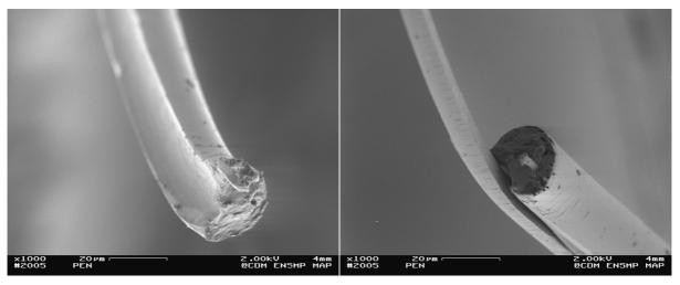
Figure 12 Complementary failure morphologies, PEN fibre, fatigue failure (0-75%), lifetime = 3.105 cycles. The failure mechanism is similar to that described in Fig.7.
