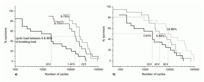
Figure 5 Lifetime data for PET fibres after different cyclic loadings.
