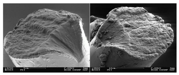
Figure 8 Complementary failure morphologies, PET fibre, cyclic loading (0-80%), lifetime = 2.103 cycles. The morphology is similar to what was previously found for tensile failures.
