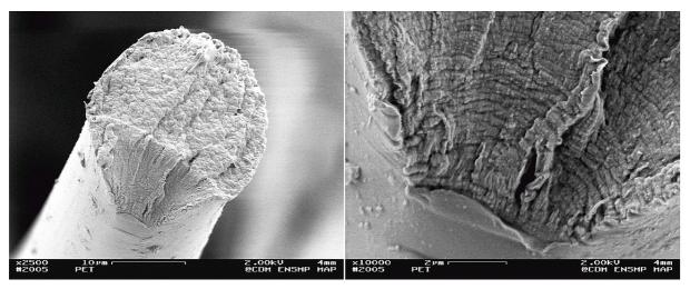
Figure 9 Failure morphology, PET fibre, cyclic loading (0-80%), lifetime = 2.104 cycles. At first sight the morphology is similar to that in Fig. 8, but a closer view of the initiation zone (right side picture) shows striations normal to the crack propagation axis.
