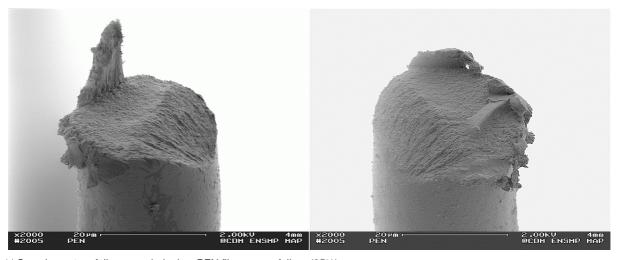
Figure 11 Complementary failure morphologies, PEN fibre, creep failure (85%).
