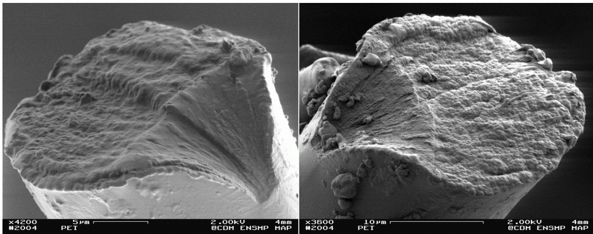
Figure 8 Complementary failure morphologies, PET fibre, cyclic loading (0-80%), lifetime = 2.103 cycles. The morphology is similar to what was previously found for tensile failures.
