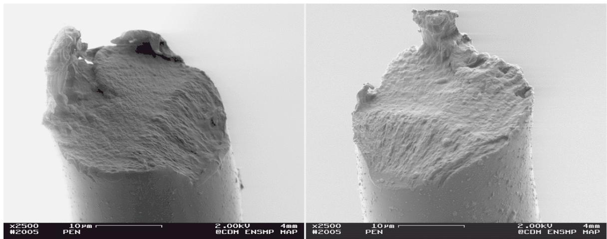
Figure 10 Complementary failure morphologies, PEN fibre, tensile failure.
