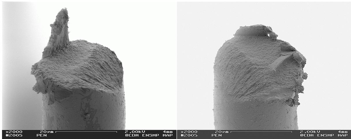
Figure 11 Complementary failure morphologies, PEN fibre, creep failure (85%).
