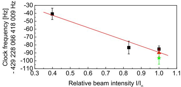
Fig. 2. Light shift due to the interrogation laser for different values of the magnetic field. ■: 1.68 mT, ▲: 1.4 mT, ★: 1.12 mT.  $I_0 \simeq 6$  W/cm<sup>2</sup> corresponds to the clock laser intensity at standard operating conditions. The line is a linear fit to the data.
