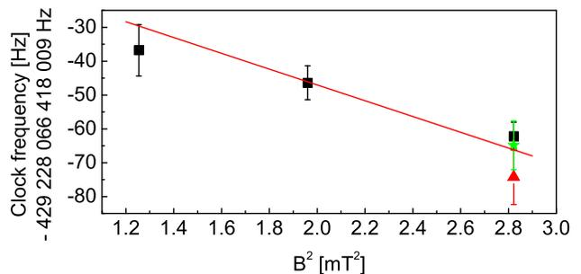
Fig. 1. Dependence of the clock frequency on the static magnetic field. The line is a fit to the experimental data with an adjustable offset, the slope being fixed to the theoretical value of Ref. <sup>20</sup> ■:  $I/I_0 = 1$ , ▲:  $I/I_0 = 0.83$ , ★:  $I/I_0 = 0.4$ .
