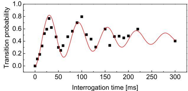
Fig. 3. Experimental observation of the Rabi oscillations for  $B = 1.68$  mT at maximum intensity  $I_0 \simeq 6$  W/cm<sup>2</sup>. The line is a fit corresponding to classical Rabi oscillations attenuated by an exponential decay. The frequency of the oscillations is  $16(1)$  Hz, the time constant of the decay is about 100ms which corresponds to the coherence time of the interrogation laser.
