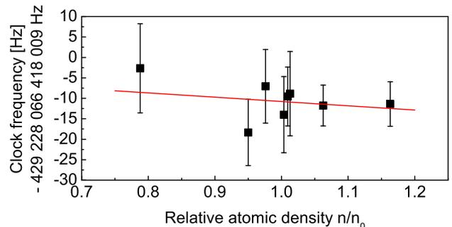
Fig. 4. Clock frequency vs atomic density. All the points have been corrected for the Zeeman and the light shifts. The line is a linear fit to the data. We have  $n_0 = 2.5 \times 10^{11}$  at/cm<sup>3</sup>.
