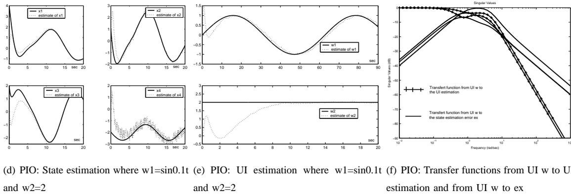
Fig. 1. State and UI estimation performance in presence of UI and actuator and sensor noises.
