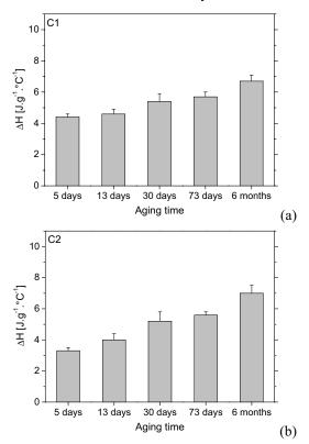
**Figure 3.** Characterization of the structural relaxation of the epoxy through DSC: enthalpy excess  $\Box$ H as a function of aging time for the composites C1 (3a) and C2 (3b).
