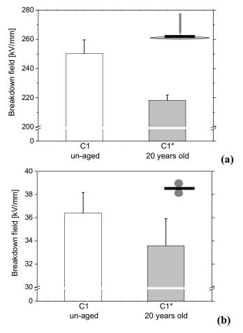
**Figure 6.** Comparative breakdown field for C1 and C1\* under divergent (a) and quasi-homogeneous (b) fields.
