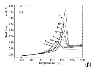
**Figure 2.** DSC Thermograms of as-received systems (a) and composites aged under laboratory conditions for (b) 9h, (c) 20h, (d) 5days, (e) 13 days, (f) 30 days, (g) 73 days, (h) 6 months – first ramp of temperature, composites C1  $(2.\Box)$  and C2  $(2.\Box)$
