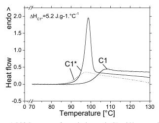
**Figure 1.** DSC thermograms of as-received composite C1 and 20-years-aged C1\*– first (solid lines) and second (dashed line) ramp of temperature.
