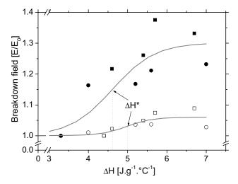
Figure 9. Normalized breakdown field as a function of enthalpy excess under divergent field for the composite  $C1 (\blacksquare)$  and  $C2 (\bullet)$  and under quasi homogeneous field for the composite  $C1 (\square)$  and  $C2 (\bigcirc)$ .
