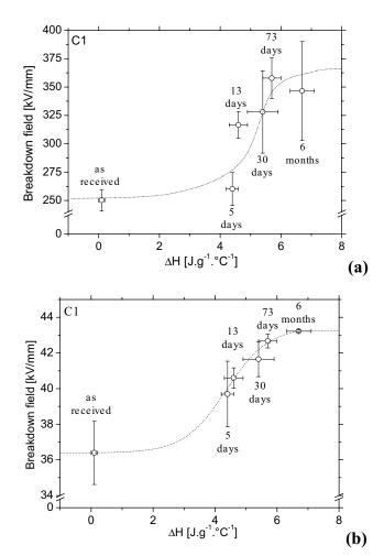
**Figure 7.** Electrical breakdown field as a function of enthalpy excess under divergent (a) and quasi homogeneous (b) field for the composite C1.
