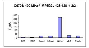
Fig. 4: MPEG2 Encoder execution time
