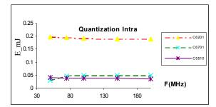
Fig. 5: Energy consumption for 3 DSP
