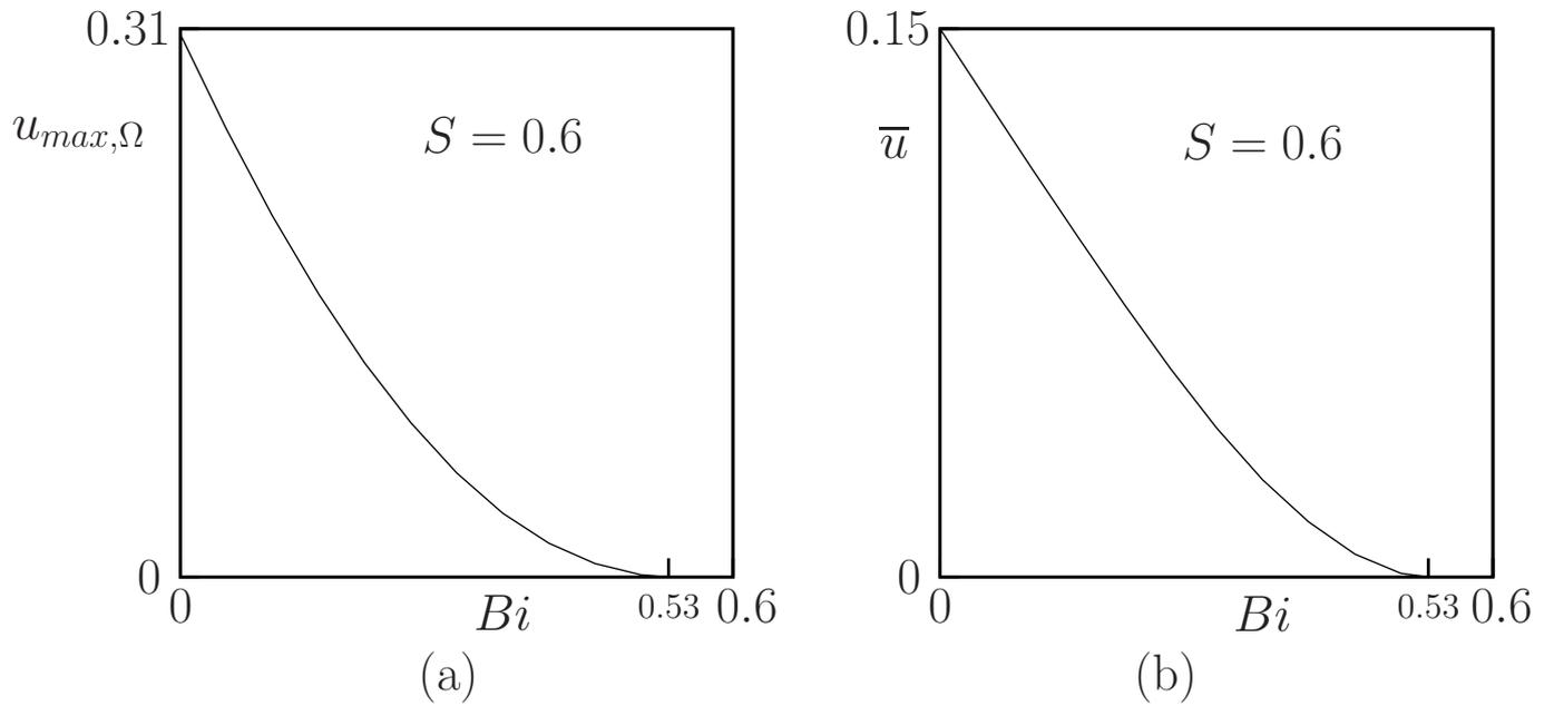
Figure 7. (a) Maximum velocity  $u_{max,\Omega}$  versus  $Bi$  for  $S = 0.6$ ; (b) Flow rate  $\bar{u}$  versus  $Bi$  for  $S = 0.6$ .
