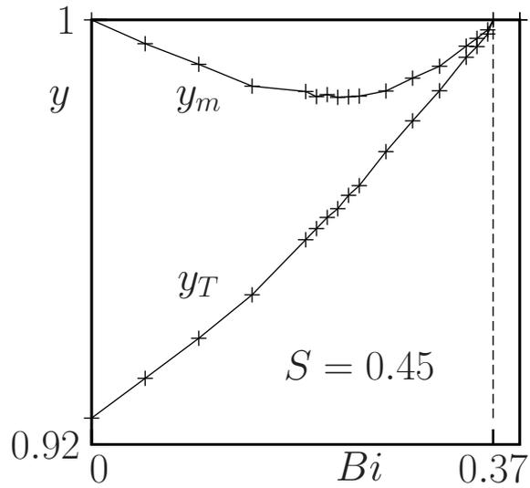
Figure 17. Position at the wall of the free boundaries as functions of  $Bi$  for  $S = 0.45$ : position  $y_m$  of the dead zone boundary, position  $y_T$  of the stick-slip transition.
