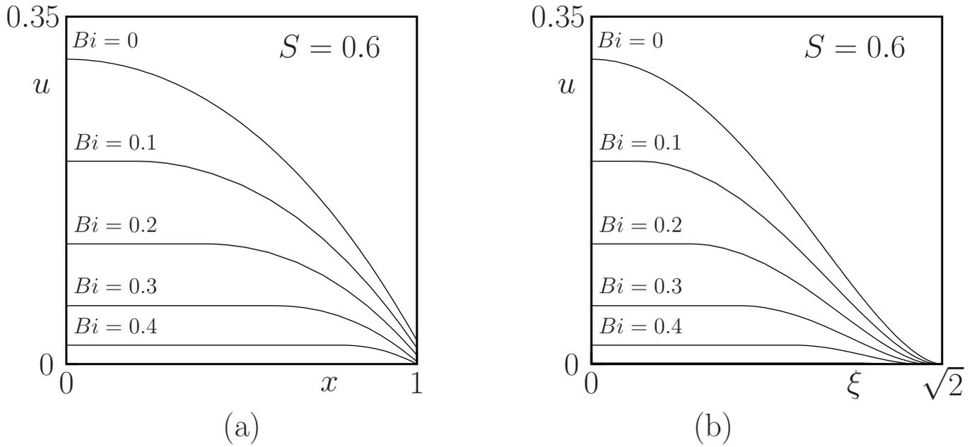
Figure 6. Velocity profiles for different values of  $Bi$  and  $S = 0.6$ : (a) cut along the horizontal axis  $y = 0$ ; (b) cut along the diagonal  $y = x$ .
