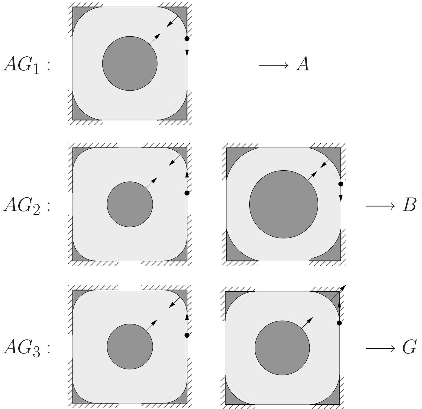
Figure 21. Schematic representation of the flow in the sub-regimes  $AG_1$ ,  $AG_2$  and  $AG_3$  when  $Bi$  increases: evolution of the rigid zones boundaries and of the stick-slip transition points.
