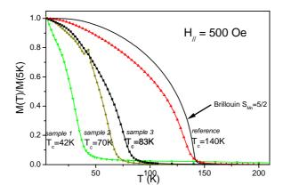
Fig. 2: (Color online) Temperature-dependence of the normalized magnetization under a 500 Oe in-plane field for samples 1-3, and reference. The solid line corresponds to Brillouin curve with  $S_{Mn} = 5/2$ , and  $T_c = 140$  K. Curie temperatures increase and curves become more convex with increasing hole density.
