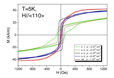
Fig. 3: (Color online) Hysteresis cycles obtained by SQUID magnetometry with the magnetic field lying in plane.
