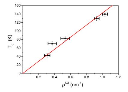
Fig. 1: (Color online) Curie temperature as a function of  $p^{1/3}$  where p is the mean hole density between n=1 and n=2 fit results (given by the tips of the horizontal bars). Full line is the fit to the mean-field expression  $T_c \alpha p^{1/3}$ .
