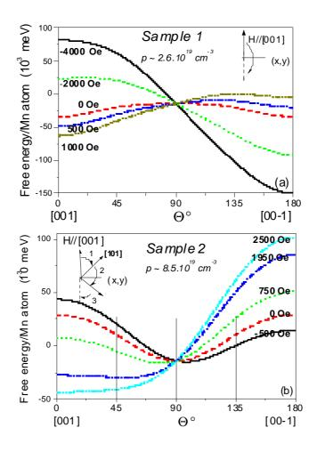
Fig. 9: (Color online) Free energy per Mn atom computed with anisotropy fields given by FMR experiments at T=4 K; the magnetic field is applied perpendicular-to-plane. At low hole densities (a), the easy axis is [001]. Upon increasing p (b), an in-plane component of the magnetization appears.
