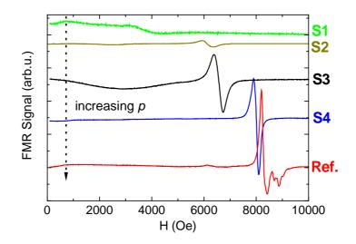
Fig. 6: (Color online) FMR spectra at T = 20 K and H//[001] for the reference sample and samples 1-4; the spectra are measured with the same gain.
