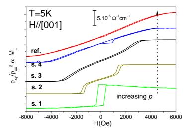
Fig. 4: (Color online) Hysteresis cycles obtained by anomalous Hall effect<sup>25</sup> with H//[001] (off-set for clarity), and assuming  $M_{\perp} \propto \rho_{xy}/\rho_{xx}^{n}$  with n=2. The magnetic easy axis flips from out-of-plane to in-plane with increasing hole density.
