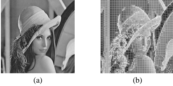
Fig. 1. (a) Original image. (b) Variable block sizes representation (subsampling grid : 0.032 bpp).
