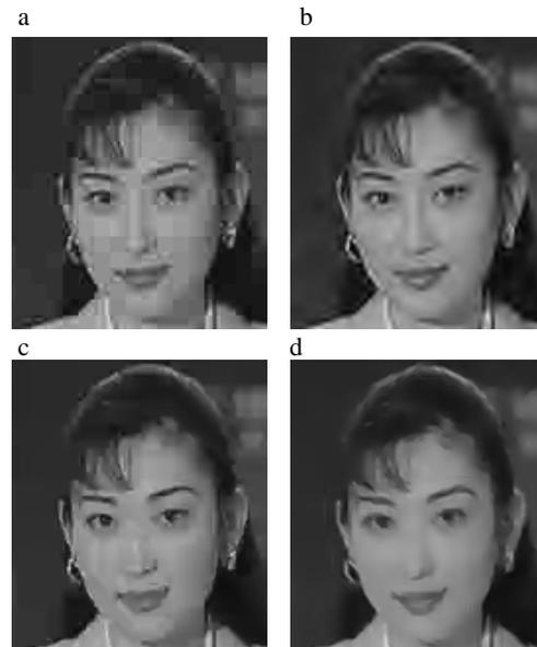
**Figure 8:** Comparative results (0.123 bpp), a) Mpeg4 b) jpeg2000, c) H.261, d) LAR
