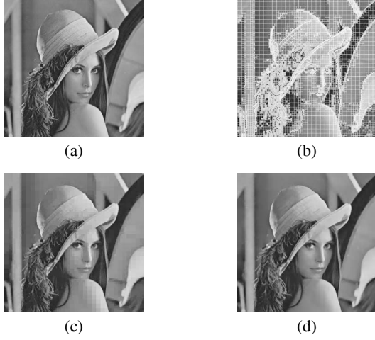
Fig. 1. (a) Original image. (b) Variable block sizes representation (subsampled grid : 0.032 bpp). (c) reconstructed low-resolution image (0.4bpp) resulting from first pyramid descent process. (d) Post-processed image.
