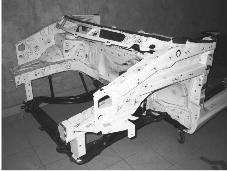
Fig. 12. Picture of cross member beam with some other constitutive parts of Peugeot 806 vehicle.
