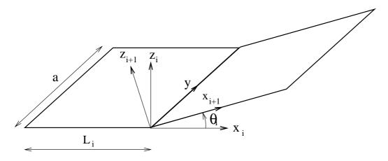
Figure 8: Notations for two coupled plates
