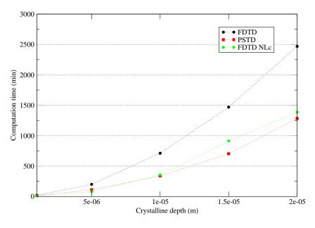
Figure 8. Computation times for the three schemes (PSTD=pseudospectral scheme, NLc=FDTD scheme of Sec. 3.3) for several crystalline lengths on an Intel<sup>®</sup> Xeon<sup>TM</sup>2.2 GHz.
