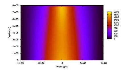
On Fig. 17, we have plotted the energy flux  $F_v$  after 400 fs.
