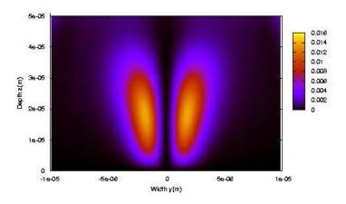
Figure 16. Energy flux  $F_x$  in a SHG experiment without phase matching after a propagation in 50  $\mu$ m of KDP (268 fs). We have used the same arbitrary units for the intensity as in Fig. 15.
