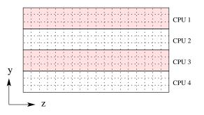
Figure 5. Load sharing between four processors.
