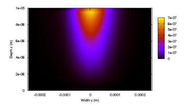
Figure 12. Energy flux  $F_x$  in a SHG experiment at the phase matching angle after a propagation in  $10 \mu m$  of KDP. We have used arbitrary units for the intensity as in Fig. 11.
