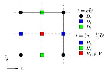
Figure 6. FDTD scheme with centered nonlinearity for the electromagnetic wave  $(\mathbf{D}, \mathbf{H})$ , the polarization **P** and the density matrix  $\rho$ .
