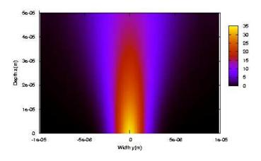
Figure 15. Energy flux  $F_y$  in a SHG experiment without phase matching after a propagation in 50 $\mu$ m of KDP (268 fs). We have used the same arbitrary units for the intensity.
