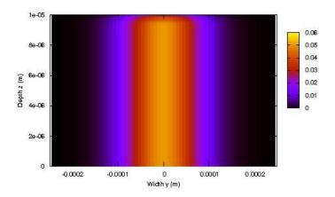
Figure 11. Energy flux  $F_y$  in a SHG experiment at the phase matching angle after a propagation in 10 $\mu$ m of KDP. We have used arbitrary units for the intensity.
