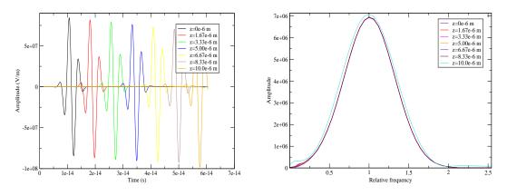
Figure 13. The  $E_y$  component and its Fourier transform in an experiment of second harmonic generation for seven points in the crystal. The amplitude of the Fourier transform is plotted in arbitrary units, the frequency is relative to the one of the incoming beam.
