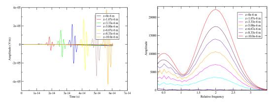
Figure 14. The  $E_x$  component and its Fourier transform in an experiment of second harmonic generation for seven points in the crystal. The frequency units of the Fourier transform is relative to the frequency of the incoming laser pulse. The amplitude of the spectrum is shown in arbitrary units.
