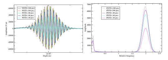
Figure 9.  $E_x$  component and its Fourier transform in an experiment of second harmonic generation using the pseudospectral (PSTD) scheme for several sizes of the space step. For comparison, we have also plotted the result obtained by the scheme of Sec. 3.1 (FDTD). The frequency is relative to the frequency of the incoming wave-field.
