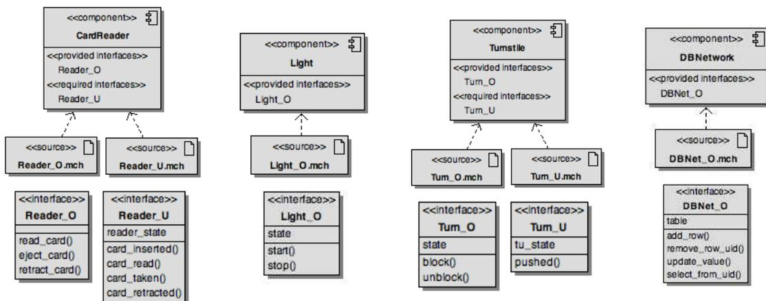
Figure 2. Les composants `CardReader`, `Light`, `Turnstile` et `DBNetwork`
